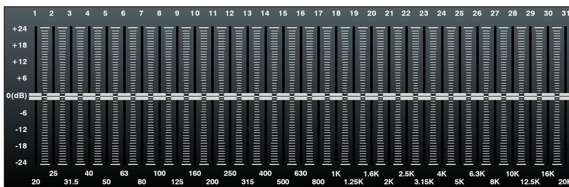
In this screen, you can adjust gain at every specific frequency. The EQ number, Frequency and Gain value which you are adjusting will be shown on the LCD below the graphic curve. Please follow the instruction that is shown on the LCD display to adjust the value.
