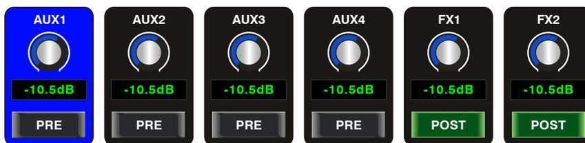
Touch AUX1-4 and FX1-2 on the LCD screen or press corresponding button on the panel to assign input channel audio to these channels or buses. To adjust output level of the channel audio, you can rotate Parameter Adjust knob on the panel.
