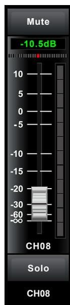
Slide the fader to change selected input channel audio. The fader function is the same with **Fader** on the panel, which can control input signal's level, they will change synchronously.
