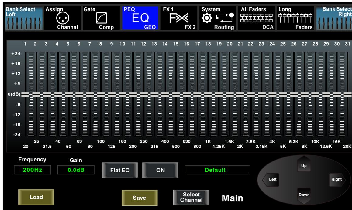
The T2208 features MAIN Stereo, AUX Mono, 31-band, 1/3 octave graphic EQs. The 31 bands range from 20Hz to 20 KHz. There is 1 MAIN Stereo GEQ, 8 AUX Mono GEQs in 24-bit/48 kHz sample rate.
