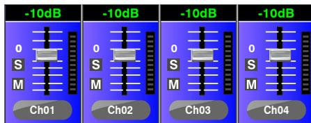
To select channels touch the box corresponding to the desired channel and that box will change color indicating that the channel was added. In the same way to remove a channel of a group, touch the channel box and this will turn off indicating their elimination.
