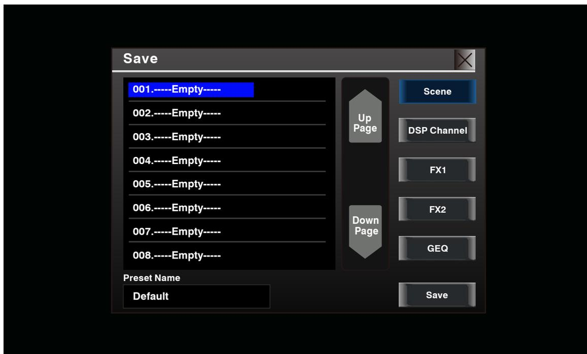
Press this button to save the selected channel's and bus's DSP channel setting as DSP presetting for future use. On the screen you can touch to save preset of DSP Channel, GEQ, DFX, Scene. Please do as the instruction that is shown on the LCD display.
