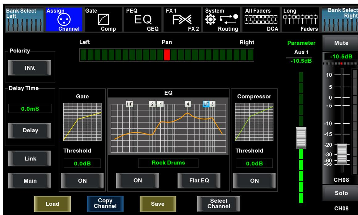
**INV.** Touch it in Polarity to invert the phase of the selected channel's signal (to alter the phase by 180°). If the phase reverse is active the button will illuminate. The LCD display shows the phase reverse setting in real time. The Polarity control can be used to correct audio signals which are out of phase as well as to cancel/reinforce each other.
