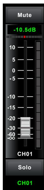
Functions on this icon (like mute, level number, pan, long fader, solo and channel name) are the same with that in Mixer interface.
