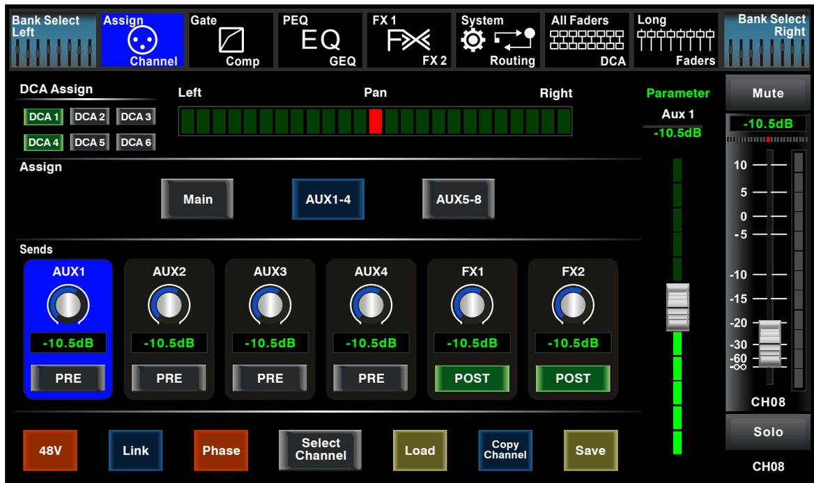
Touch Main AUX1-4 on the LCD screen or corresponding button on the panel to assign input channel audio to these channels or buses. They will illuminate synchronizing with buttons in Assign area on the panel after pressed. To adjust output level of the channel audio, you can rotate Parameter Adjust knob or corresponding Main or AUX1-4 knobs on the right corner of the panel.
