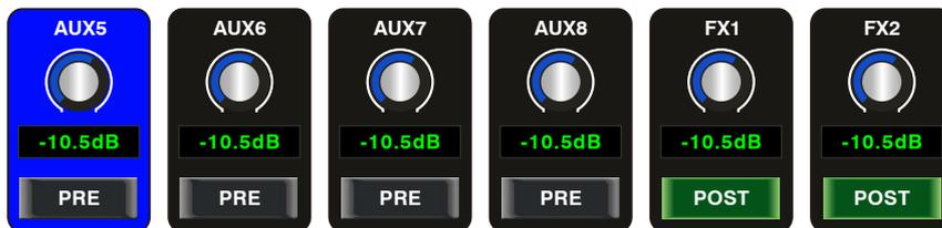
Touch AUX5-8 and FX1-2 on the LCD screen to assign input channel audio to these channels or buses. To adjust output level of the channel audio, you can rotate Parameter Adjust knob on the panel.
