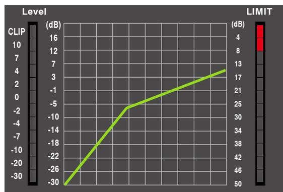
The compressor grid shows level setting of threshold in real time.
