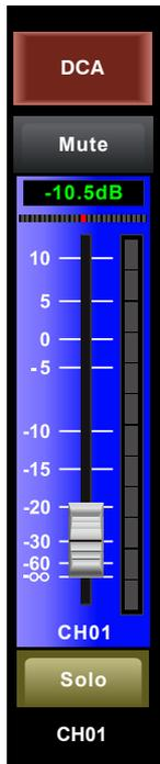
Meter beside the fader indicates the input signal level activity. This long fader can control level of all input and output channels in this screen, but for one selected channel at one time, all its control will change synchronized with the selected channel.
