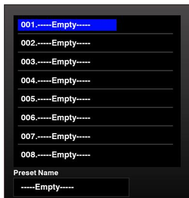
This items show names of preset, when you select a preset, its name will show on the bottom box, then touch Load control on the right corner of the screen to load the selected preset to corresponding controls.
