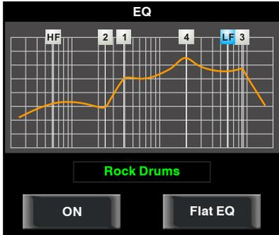
Touch the switch ON to enable EQ function, it will illuminate and synchronize with ON/OFF control in EQ page. Please set values in EQ page because it is not adjustable here. This page can only show the values. You can also load a preset, please refer to load introduction section for the detail operation, the loaded state will show in the middle box.
