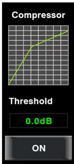
Touch the switch to enable Compressor function, then rotate Parameter Adjust knob or slide long fader on the right LCD screen to adjust value of Threshold, which will show in the middle box. During adjustment, corresponding figure change will show in the Compressor grid.
