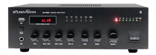
**The SA-60BT** USB/BT Portable Mixing Amplifier Compact provides 60 watts of output power with Bluetooth, integral USB audio player power, and 5 inputs including 3 balanced MIC (MIC1 has another port of 6.35mm jack on front panel), 2 unbalanced AUX, each one has individual volume control.
