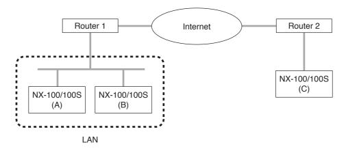
Connections can be made from Unit C to Unit A using the global IP address. The global IP address used for the connection is converted into the local address for Unit A by Router 1.
