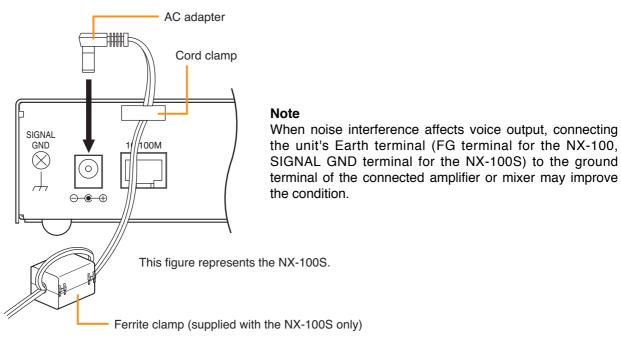
Mount the ferrite clamp (supplied with the NX-100S) on the cable in a way that the cable is looped one turn as illustrated. (This countermeasure is for complying with the CE marking requirements.)
